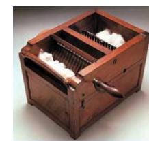
Eli Whitney patented the cotton gin on March 14, 1794. The cotton gin is a machine that separates seeds, hulls and other unwanted materials from cotton after it has been picked.
